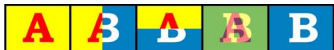
A INPUT, L/R SPLIT MODE, T/B SPLIT MODE, FADE MODE AND B INPUT
